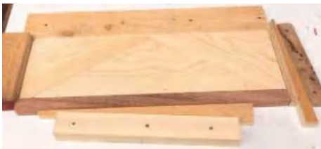
▲ Pic.6 Here you can see the first results of a carcass panel, which I glued up in a custom-made jig. It came out really well and the jig works a treat. I then went on to load a second panel so that I could practise my 'SunRay Dovetails' on them
